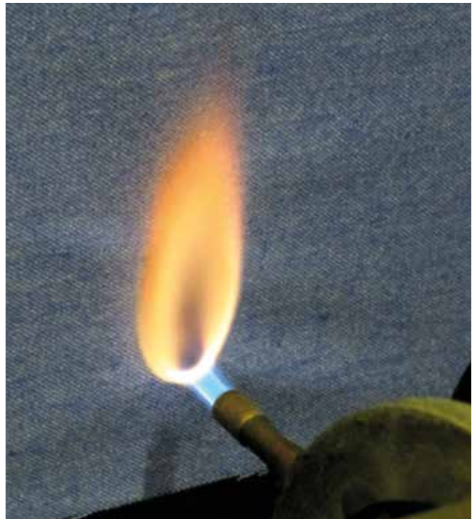
Above: Flame being applied to fabric during BS 5867 Part 2
